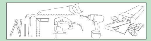
When cutting the Pergo wood plank be sure you are not creating splinters or chipping when cutting. If using a handsaw keep the decorative surface faced up. If using a jigsaw keep decorative surface down.
