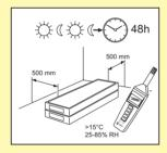
Installing in winter time in very low RH, the clearance should lowered to 8 mm (low RH = floor shrinks). If installing in summer time with a high RH level the clearance should be raised to 15 mm (high RH = floor expands). The clearance should be
