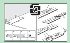
Narrow down the width of the first row or as a minimum cut off the tongue to achieve the first distance to the wall. If the wall is curved/uneven the first row has to be cut and coped to the contour of the wall. Use spacers! Cut off the tongue on the first plank also on the short side. This plank will then have the plastic tongue in the end to the right side.
