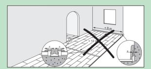
Before starting carefully measure the length and the width of the room to pan a precise lay-out to achieve a balanced appearance of the floor. This will ensure also you won't end up with the last row being too narrow. If the last row would be less than 40 mm the installation will be easier if you cut down the planks of the first row in the width.
