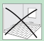
In a glued installation you have no length and width restrictions. An expansion gap around the perimeter of the room is still obligated but a T moulding in the doorways is not necessary anymore.
